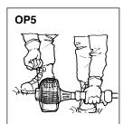
5. Firmly grasp (a) and (b) with left hand, pull the starter knob quickly until engine fires. (OP4,5)
